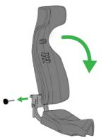
$\begin{array}{l} 1 \\ \text{Remove thumb screws and fold down} \\ \text{the seats behind buoyancy panels A} \\ \text{and D} \end{array}$
