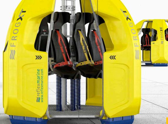
SPRING SUSPENSION SYSTEM HIGH PERFORMANCE COIL SPRINGS
