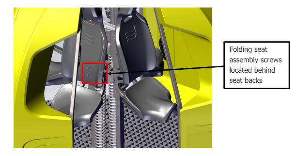
Remove the screws one at a time and replace with the longer M10 socket head screw and spring washer. Take care not to cross thread the screw.
