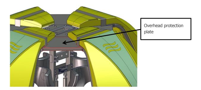
Remove the bolt and plain washer one at a time and then refit including the spring washer. Take care not to cross thread the bolt.
