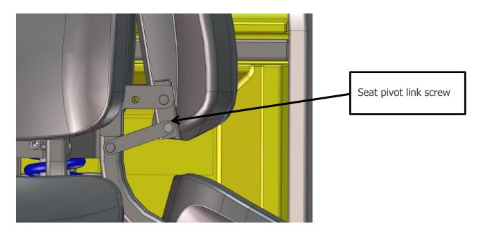
In order to fit the spring washer, remove the bolt as shown and refit the bolt with the spring washer in place. Take care not to cross thread the bolt.
