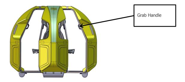
Remove the two screws securing the grab handles and refit securely including a spring washer. Take care not to cross thread the screws.
