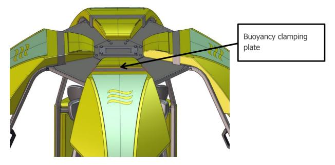
Each clamping plate is secured in place with two screws and two plain washers. Remove each one, one at a time, then refit including the spring washer. Take care not to cross thread the screw.
