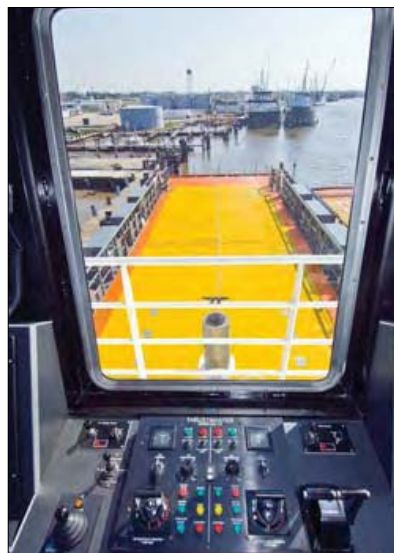
Figure 10. View from the wheelhouse providing excellent visibility for deck operations and station keeping
