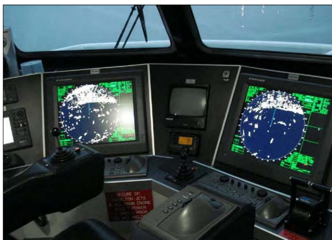
Figure 7. Seacor Cheetah is equipped with state-of-the-art navigation equipment and steered with joystick control
