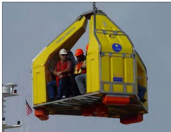
Figure 2. Frog 9 High Capacity Transfer Capsule
