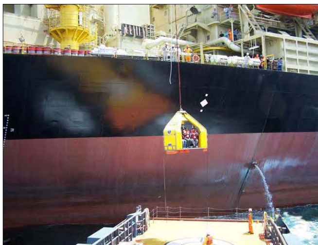
Figure 16. Frog 9 Transfers underway at the FPSO Gimboa
