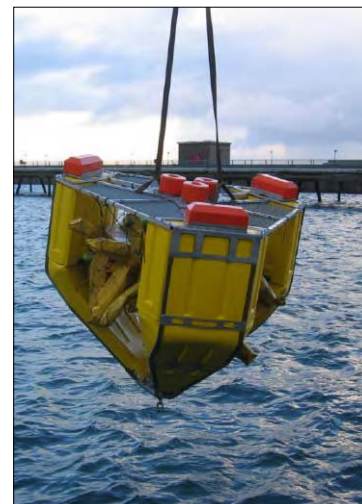
Figure 13. Frog 9 undergoing immersion testing
