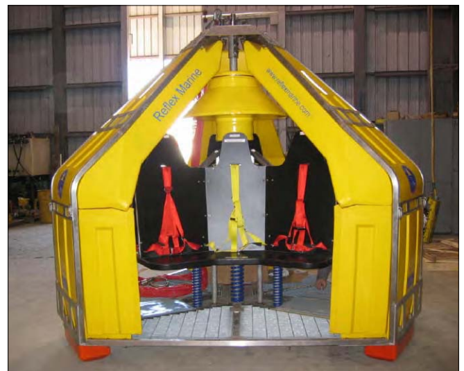
Figure 6. The first production model Frog 9 - clearly showing seat restraint
