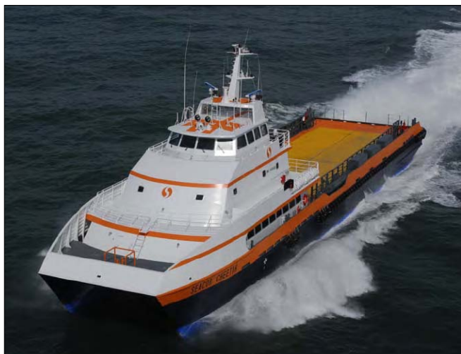
Figure 1. Seacor Cheetah - Advanced crew supply with a top speed over 40 knots
