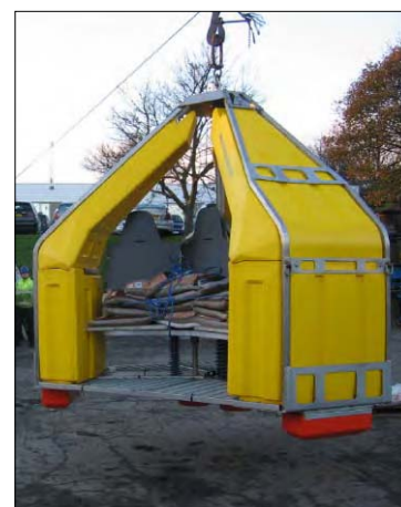
Figure 12. Frog 9 undergoing drop testing
